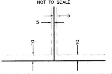
BEING 5 FEET IN WIDTH AND ADJOINING LOT LINES, UNLESS OTHERWISE INDICATED, AND 10 FEET IN WIDTH UNLESS OTHERWISE INDICATED AND ADJOINING RIGHT-OF-WAY LINES, AS SHOWN ON THE PLAT
