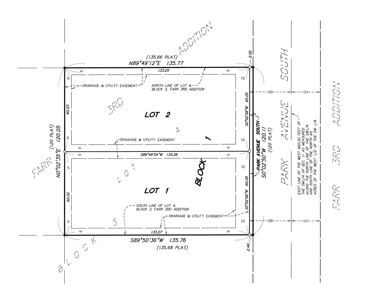
For the purposes of this plat, the north line of Lot 4, Block 3, FARR 3RD ADDITION is assumed to have a bearing of N89°49'12"E.
